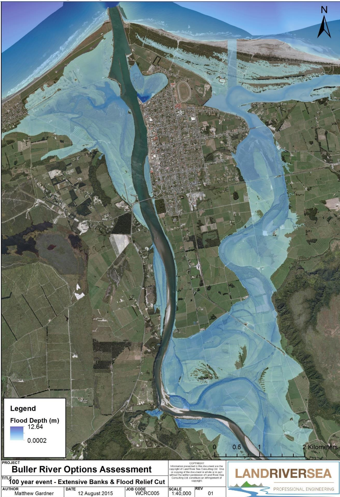
Figure A-10 - 100 year flood extent / depths - Option E – Extensive Stopbanks & Flood Relief Cut
