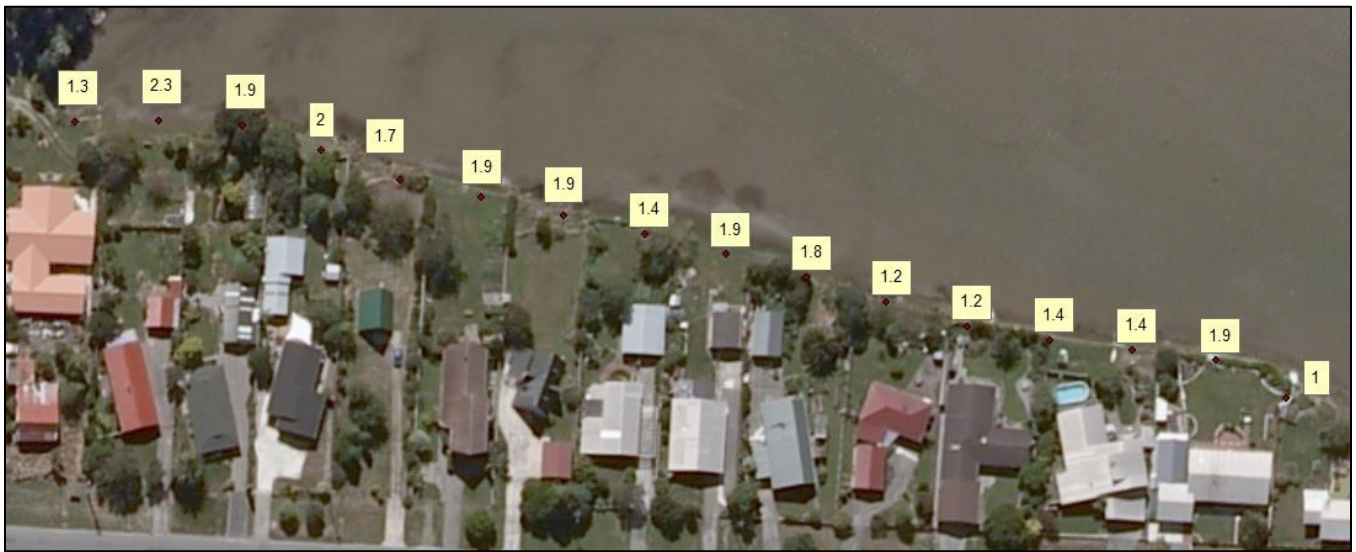
Figure 6-2 –Floodwall design heights along the Orowaiti Lagoon for a 50 year event with Option E
