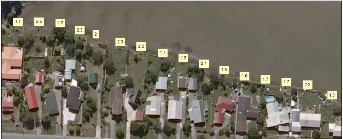
Figure 6-1 –Floodwall design heights along the Orowaiti Lagoon for a 50 year event with Option B
